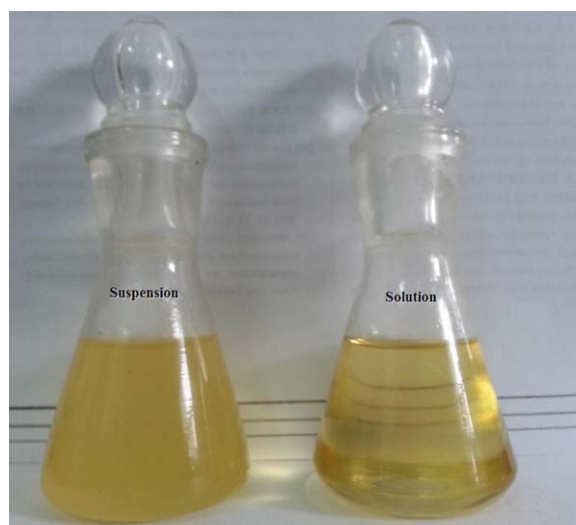
Figure 1. The appearance of suspension and solution of mulberry wood in TEACl/DMSO with dissolution condition of TEACl at 20 wt %, temperature at 40°C and stirring time for 3 h. [Color figure can be viewed in the online issue, which is available at wileyonlinelibrary.com .]
